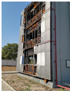
IIT-G Exterior Wall Fire Test, simulated Grenfell Tower Fire. FCIA Photo
